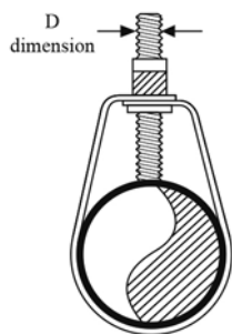
Adjustable swivel Ring-rod tight to pipe
